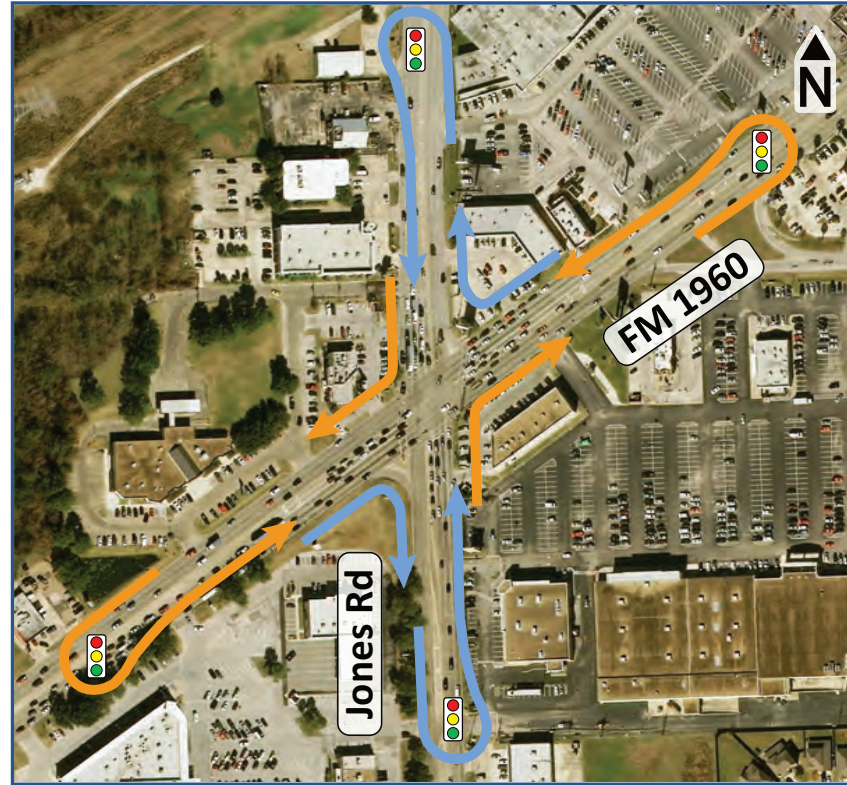
Median U-Turn Intersection
