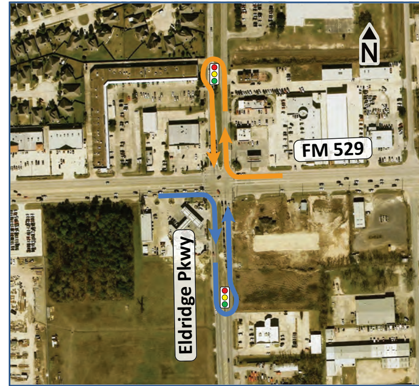
Median U-Turn Intersection
